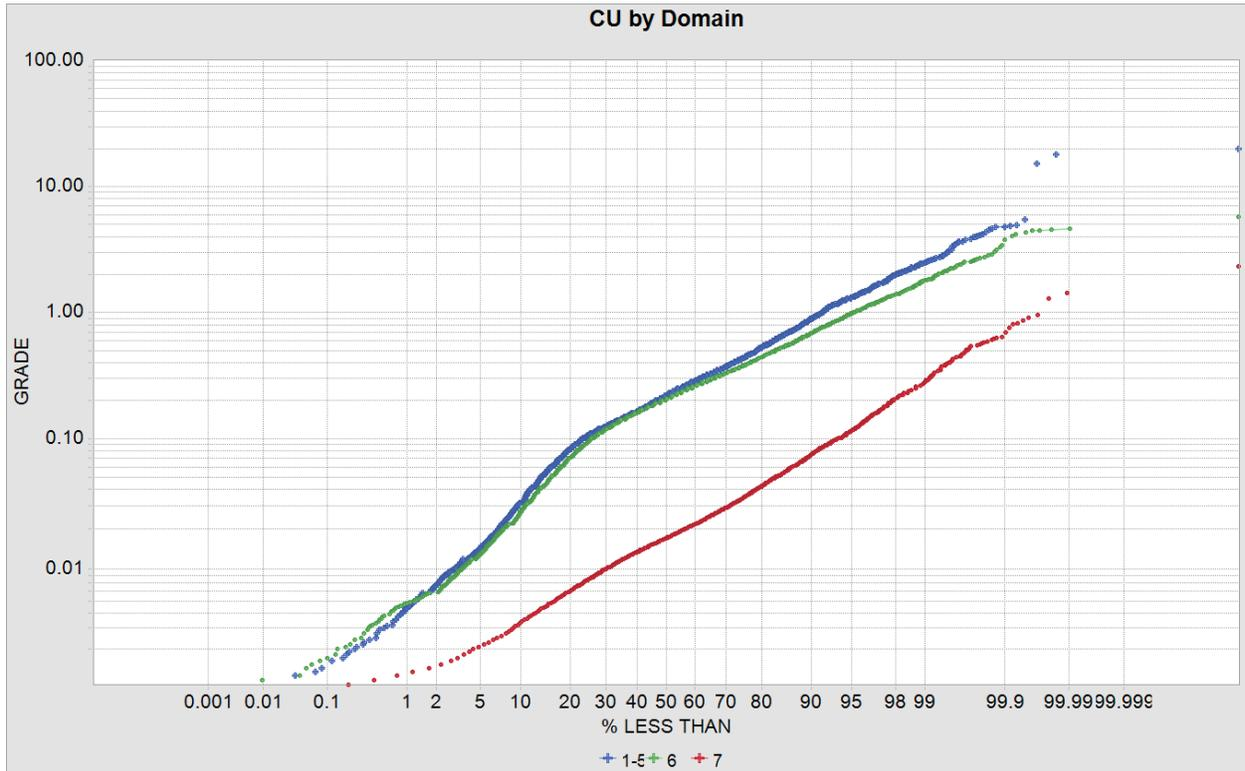
**Figure 14-9: CPP of the Cu Grade Distribution by Domain**
