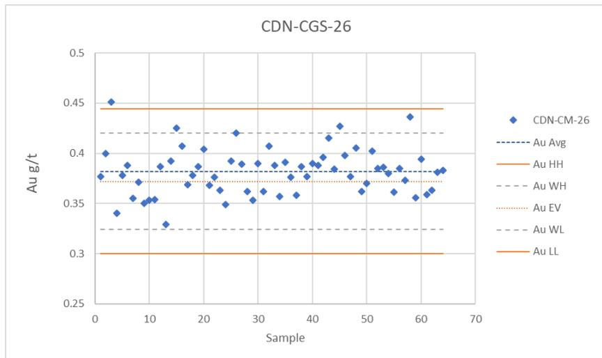
**Figure 12-7: Process Control Chart for CDN-CGS-26 Au**
