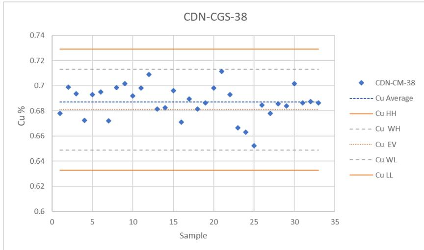
**Figure 12-3: Process Control Chart for CDN-CGS-38 Cu**
