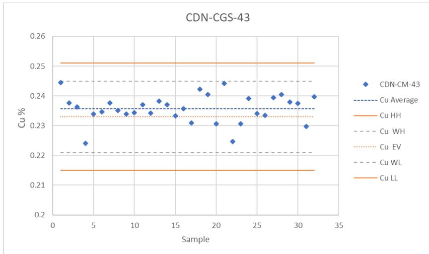
**Figure 12-6: Process Control Chart for CDN-CGS-43 Cu**
