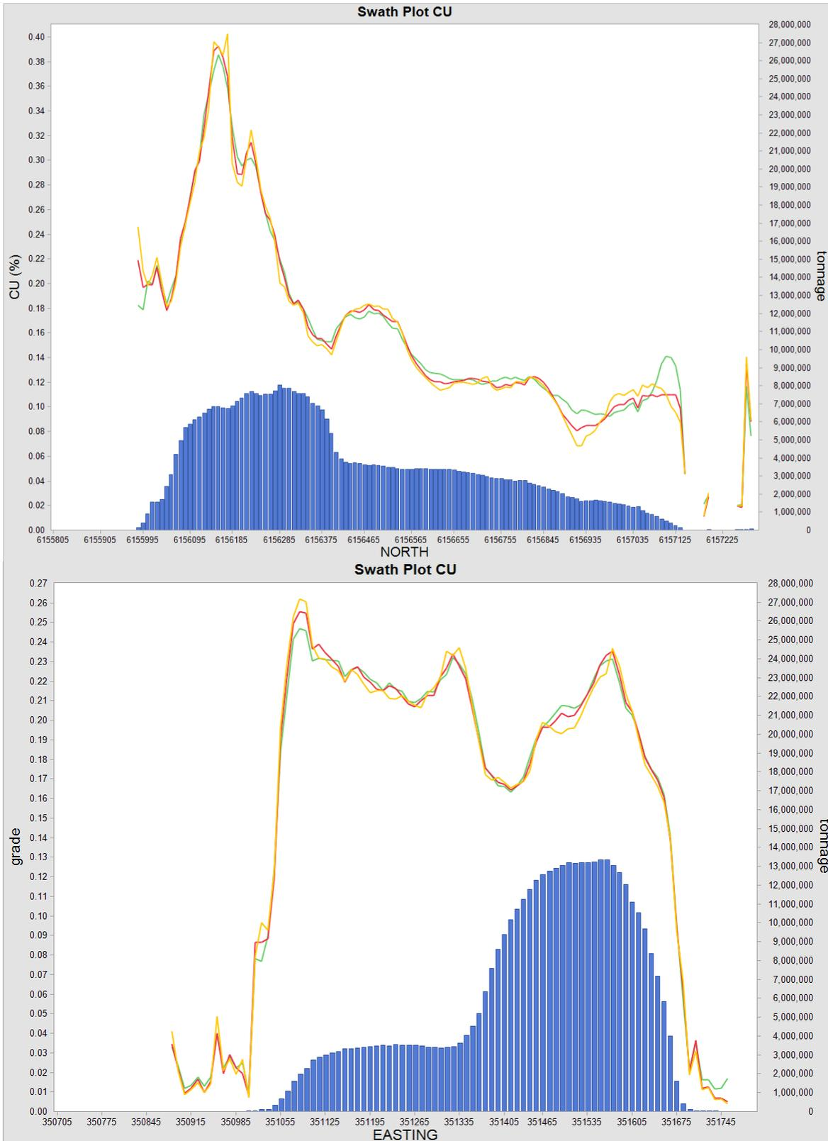
**Figure 14-15: Swath Plots for Cu – MI Classification – Central Zone**
