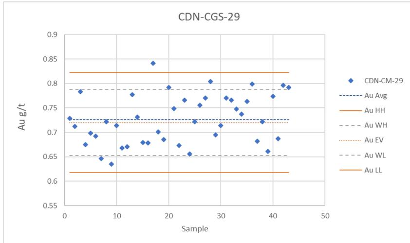
**Figure 12-8: Process Control Chart for CDN-CGS-29 Au**
