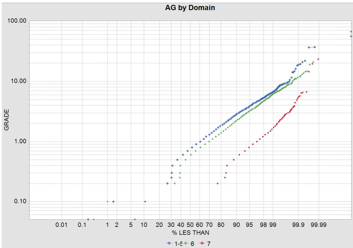
**Figure 14-11: CPP of the Ag Grade Distribution by Domain**
