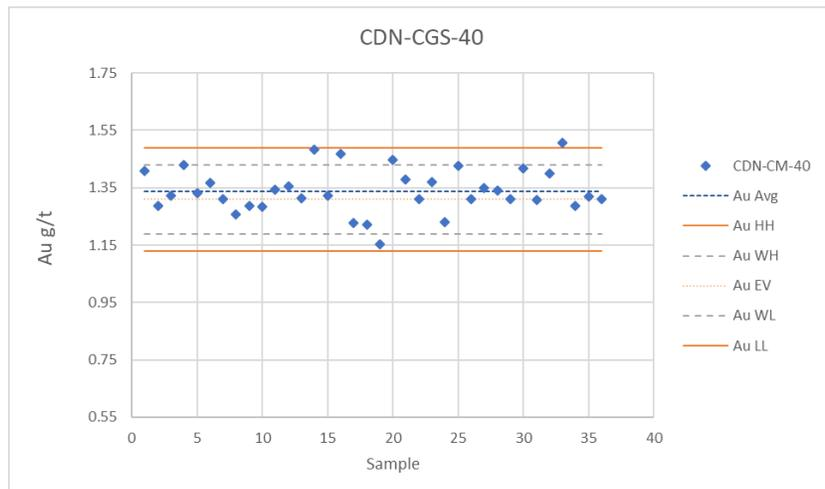
**Figure 12-10: Process Control Chart for CDN-CGS-40 Au**
