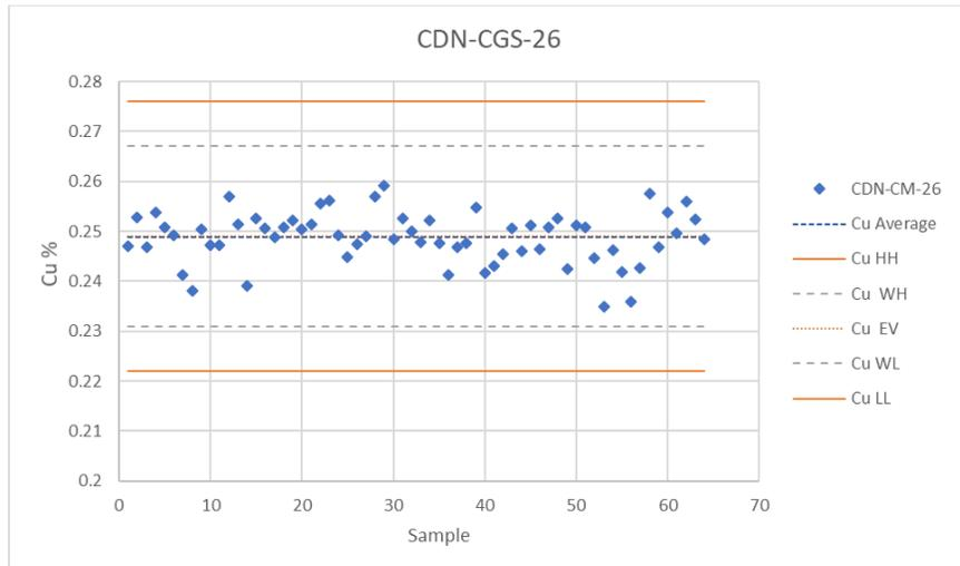
**Figure 12-1: Process Control Chart for CDN-CGS-26 Cu**
