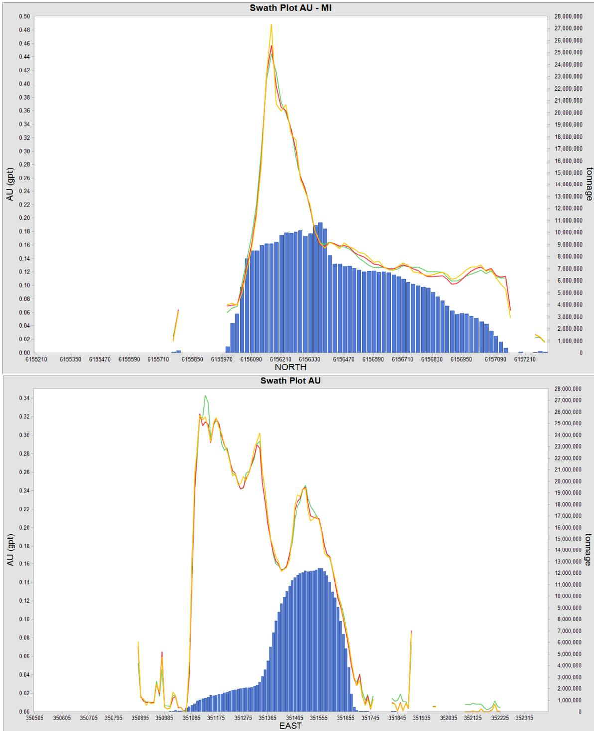
**Figure 14-16: Swath Plots for Au – MI Classification – Central Zone**
