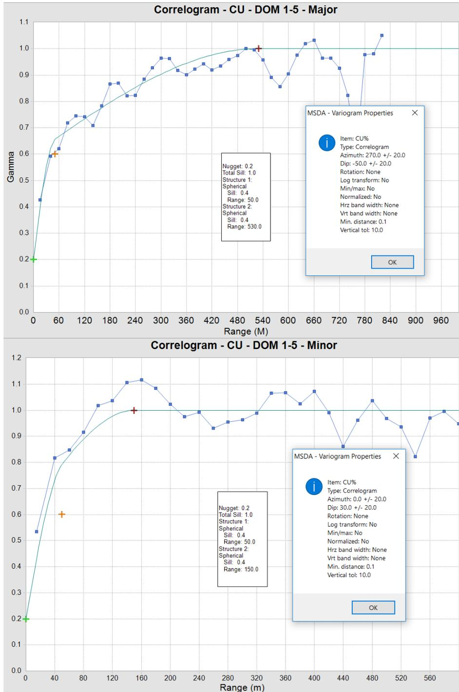
**Figure 14-12: Variography for Cu – Domains 1-5 – Major and Minor Axes**
