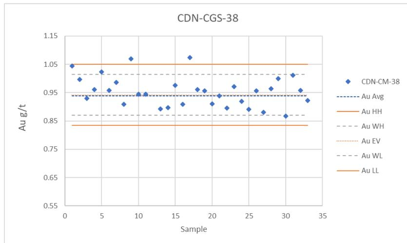
**Figure 12-9: Process Control Chart for CDN-CGS-38 Au**
