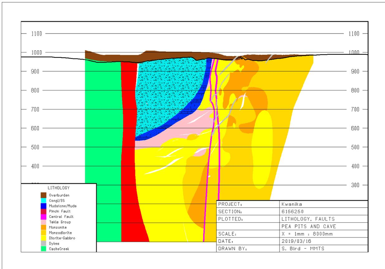
**Figure 14-2: Lithology used in Resource Modelling – Section 6156250N**
