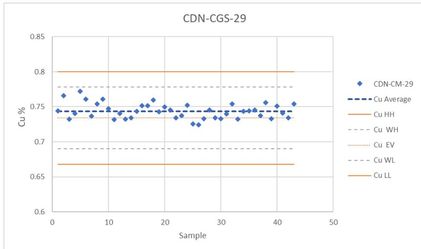
**Figure 12-2: Process Control Chart for CDN-CGS-29 Cu**
