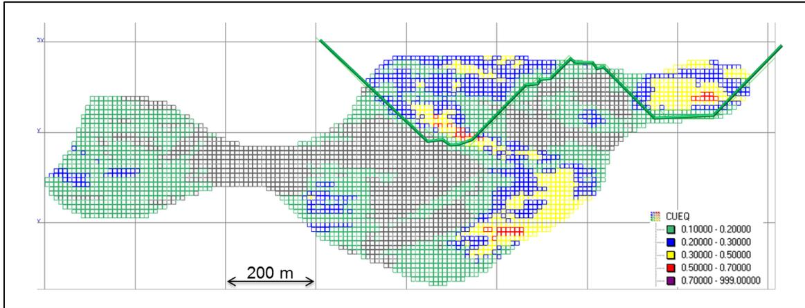
**Figure 14-25: South Zone: North-south 352,390E section of the Whittle Shell and Estimated Copper Equivalent Block Grades**
