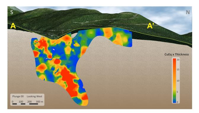
Figure 3 - Long Section Showing CuEQ % x Thickness (m)
